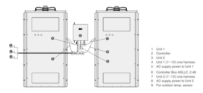
Free cooling operation condition: When outdoor temperature is ok, the two units will work simultaneously. It will minimize the energy consumption to supply maximum cooling capacity by using EC fan.
